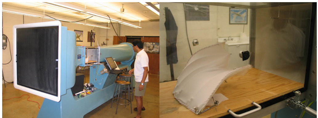
Figure 10 Physical wind tunnel testing and deflection (shown at 50 mph), after model by Knowles
